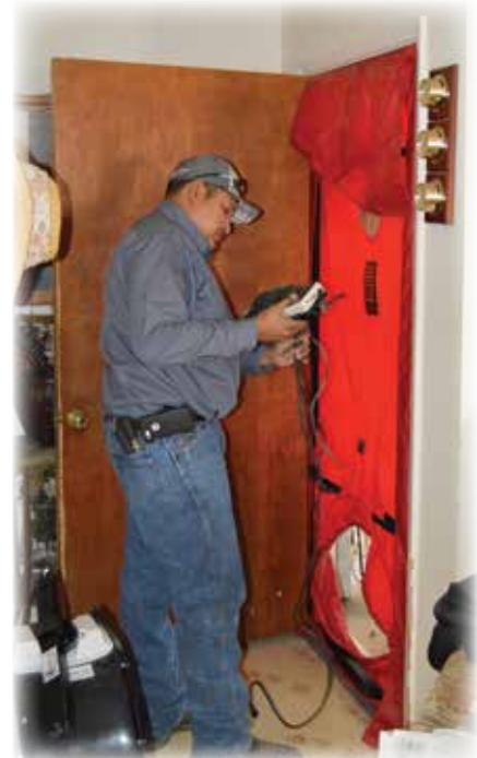
Professional home energy auditor looks at results from the blower door test that measures the airtightness of a home.
